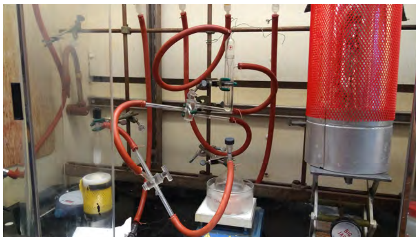
Figure 3.31 Photo of the experimental setup used to hydrogenate (–)-terpinen-4-ol with the hydrogen generated from the preparation of [TBA]2.
